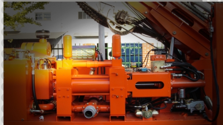
Deep hole drilling/D&B-1500MP(1500ℓ/min)
