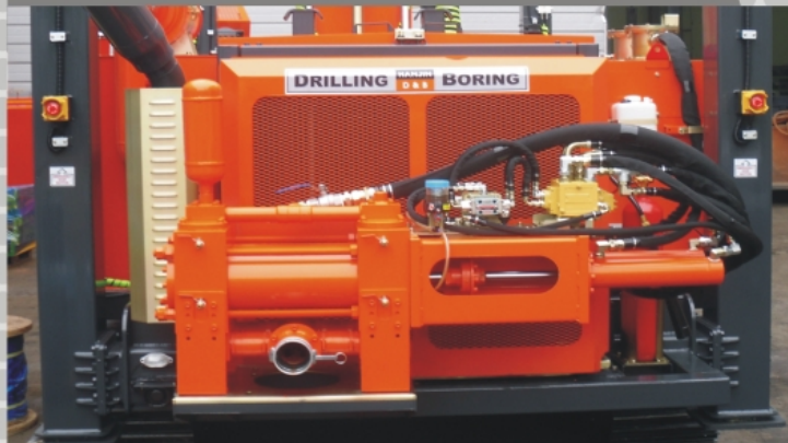
Diamond core drilling/D&B-1200MP(1200ℓ/min)
